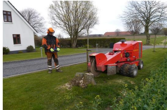
All travel and stump grinding operations are controlled via the radio remote control. A battery charger with a spare battery for the radio control system is mounted on the machine. Includes a cable to connect directly to the remote control.
